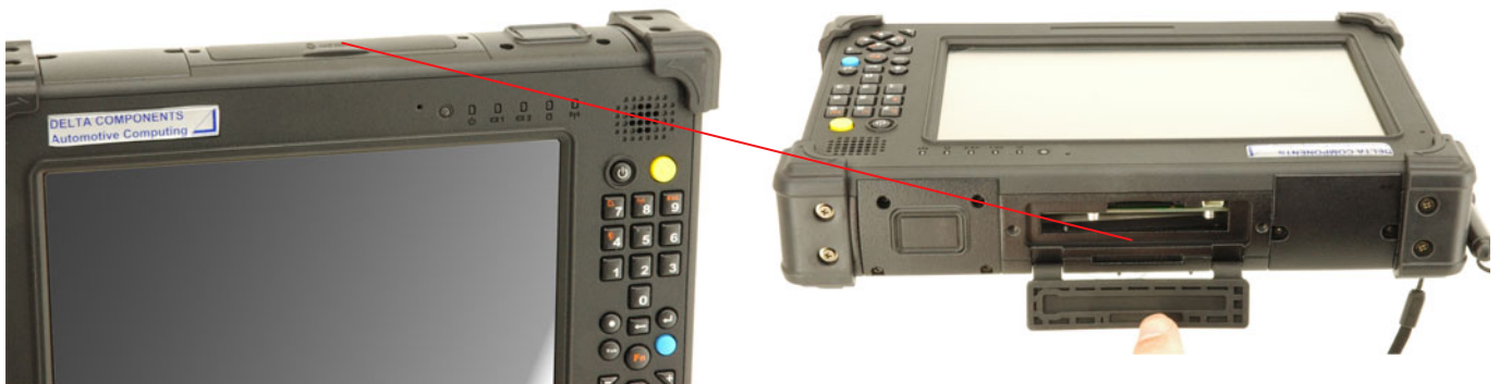
Right view: Serielle port (RS232), RJ45 port, USB port
