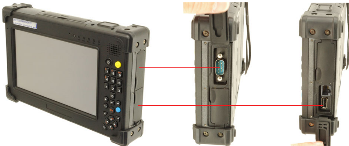
Right view: Serielle port (RS232), RJ45 port, USB port
