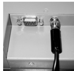
Screw-type power input
