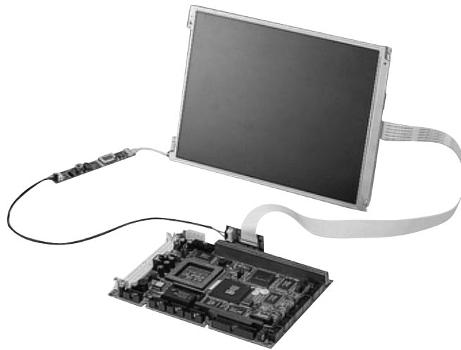
Photo 1.2 - Install the SBC-side adapter to the proper LCD interface on the AXIOMTEK SBC.
