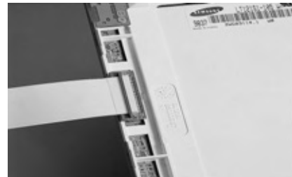
Photo 4 - Connect the inverter cable from SBC-side adapter to the inverter.
